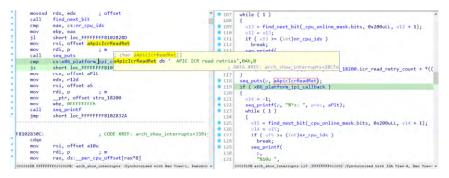
We can see a string literal is displayed as a variable name (aApicIcrReadRet) even though it is a nice-looking string in the disassembly. The mystery can be cleared up if we jump to its definition (e.g. by double-clicking) and inspect the segment properties (Edit > Segment > Edit Segment..., or Alt - S). We can see that the segment is marked as writable:
