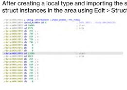
To extend the struct, press \* and enter full size. For example, the first one should be 14 (8 for the fixed part and 6 for ".text" and terminating zero), although you can also use the suggested 16:
