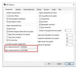
Whenever IDA outputs an instruction operand with the numerical value in that range, and it does not yet have an explicitly set type (i.e. it has the default AKA void type), it will use a special color (orange in the default color scheme):
