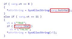
However, for the other reference the iVal filed was selected. While it is compatible for the use case (comparing against zero), by looking at the code it's obvious that the code is interpreting a boolean variant value (this can be made more clear by replacing the number 11 by the symbolic constant VT\_BOOL). This means that boolVal is a more logical choice, and we can pick it by using "Select union field..." from the context menu, or the same Alt-Y hotkey as for disassembly.
